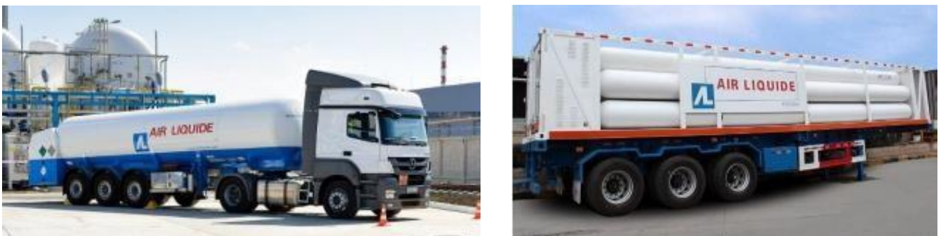
Figure 4 - Air Liquide LH 2 trailer (left) and GH 2 tube trailer (right) [8]
