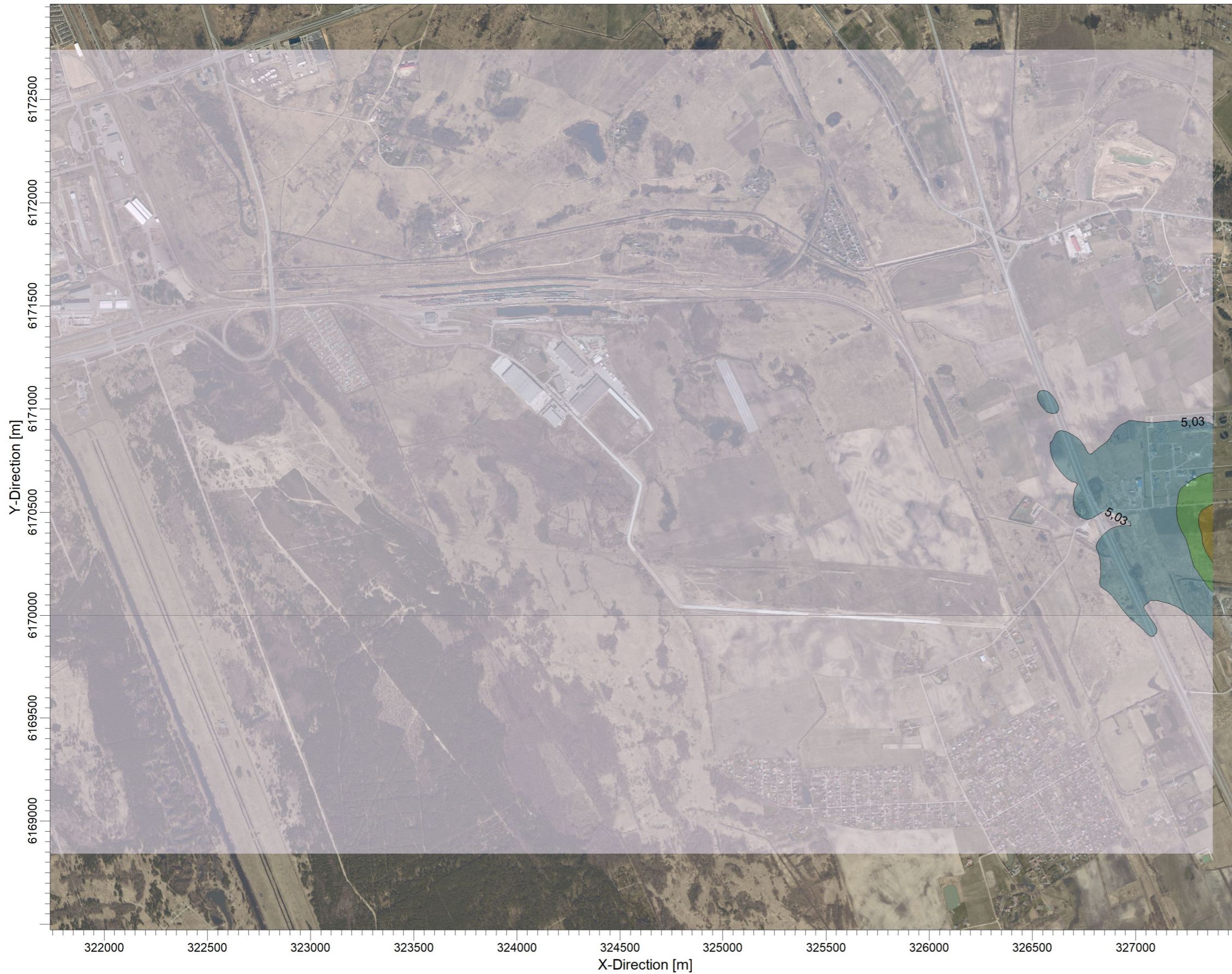
PLOT FILE OF ANNUAL VALUES AVERAGED ACROSS 5 YEARS FOR SOURCE GROUP: KD25 Max: 5,11 [µg/m³] at (327374,97, 6170341,81)
