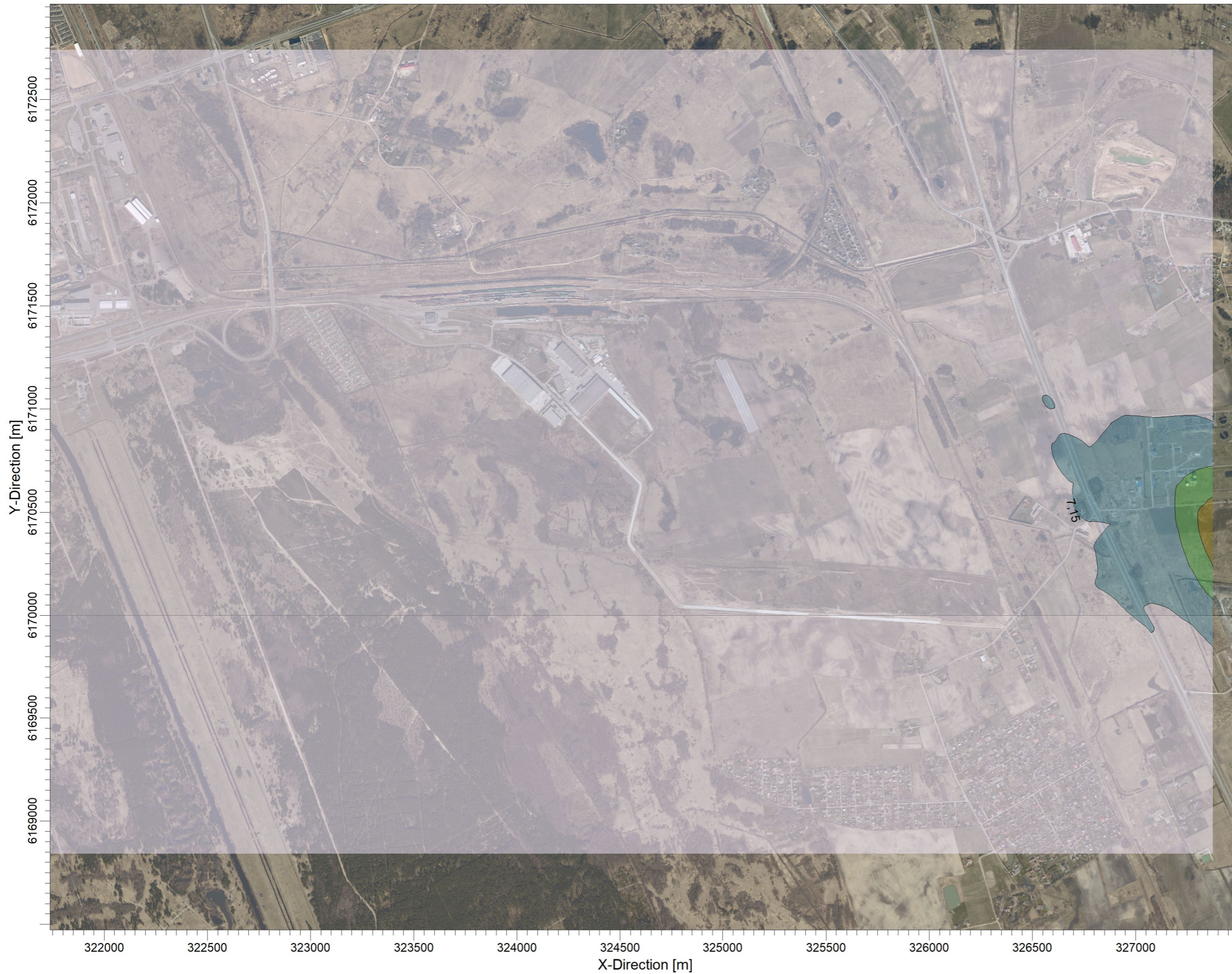
PLOT FILE OF ANNUAL VALUES AVERAGED ACROSS 5 YEARS FOR SOURCE GROUP: KD10 Max: 7,29 [µg/m³] at (327374,97, 6170441,81)
